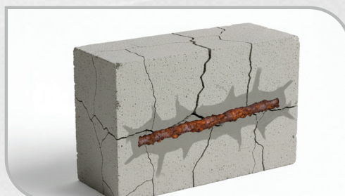
Concrete Cracks & Spalls
